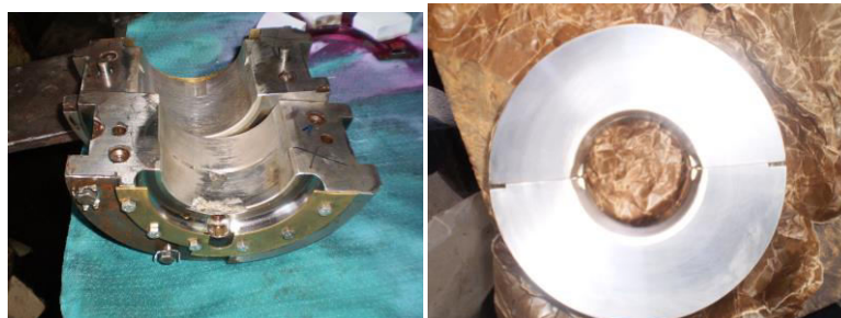
Figure 8. Damage to the plain bearing (left) and the appearance of the new "lemon" bearing (right).
